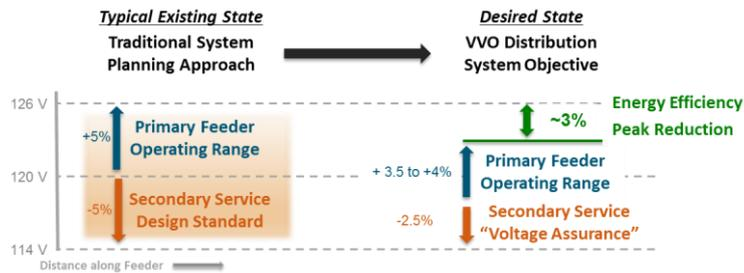
**Figure 2. Achieving VVO Objectives means modifying primary and secondary operating voltage range standards**
