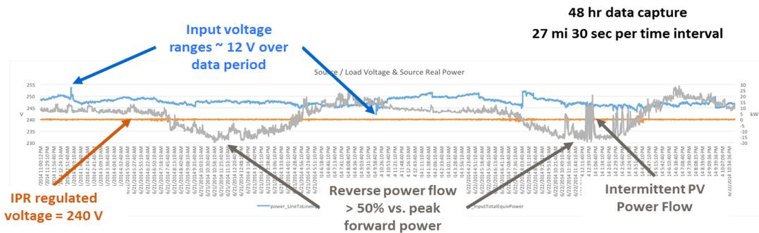
Figure 9. A data snapshot showing source voltage (blue), IPR output (load) voltage (orange) and power flow (gray). The y-axis scale to the left is voltage and the IPR setpoint is 240 V. The scale to the right is real power flow. During the highest solar production time of each day, the secondary circuit has reverse power flow of more than 50% of the highest daily load. The power electronic based IPR is regulating voltage consistently throughout the entire period.
