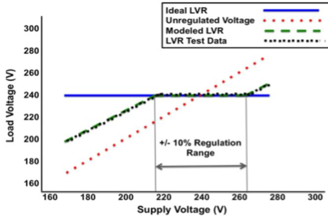
**Figure 5. Lab test results validating regulating characteristic of the LV IPR.**
