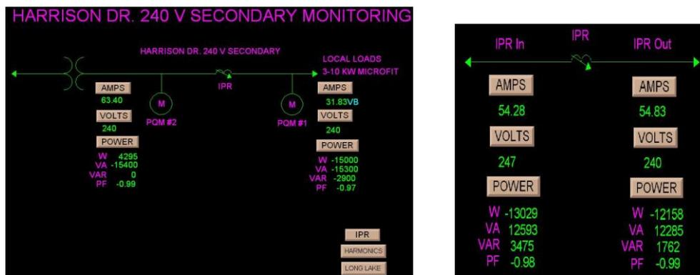
**Figure 8.** The screen shot to the left shows PQ readings for a case with the IPR output voltage and input voltage both being equivalent at 240 V and the IPR providing 2.5 kVAR. In the right half of the figure, the data from the IPR's onboard monitoring system show that the device is regulating a 247 V input voltage to the setpoint of 240 V and providing a fixed 2.5 kVAR.
