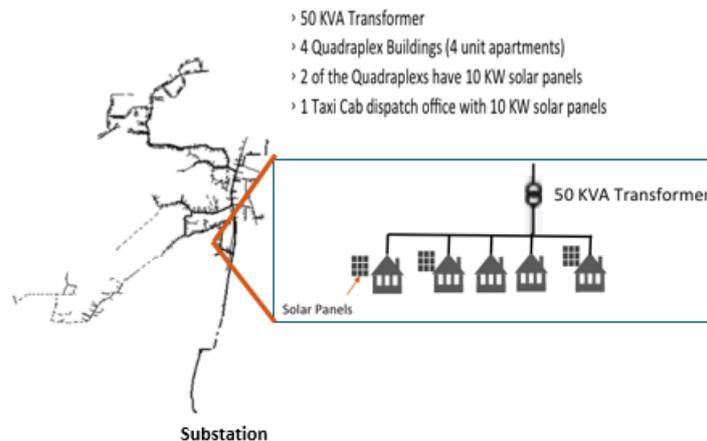
**Figure 6. An overview of the feeder circuit topology and the secondary detail prior to the IPR trial.**
