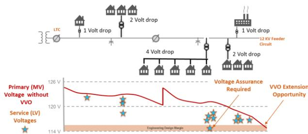
**Figure 3. Voltage Assurance and VVO Extension are two mechanisms for using the regulating capability of LV IPRs to generate feeder level Peak Reduction and EE.**
