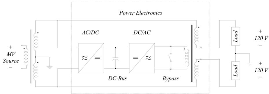
**Figure 4. UPFC architecture of the power electronics in line power regulator.**
